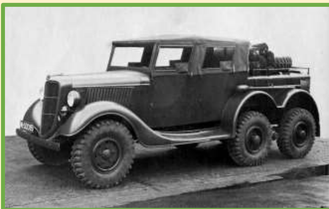
Ford based TRADO (DAF) 6 x 4 artillery tractor, DAF converted Ford 4x2 truck to a 6x4 off road capable vehicles. It was produced in a range of cab styles with seating from 6-12.
