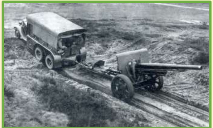
Ford based TRADO (DAF) 6 x 4 artillery tractor, DAF converted Ford 4x2 truck to a 6x4 off road capable vehicles. It was produced in a range of cab styles with seating from 6-12.
