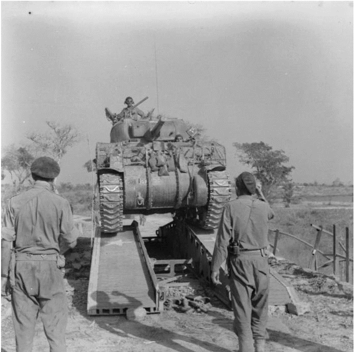
Above: A Sherman of 9th (Royal Deccan) Horse crosses a Valentine AVLB-laid bridge near Meiktila in 1945.
